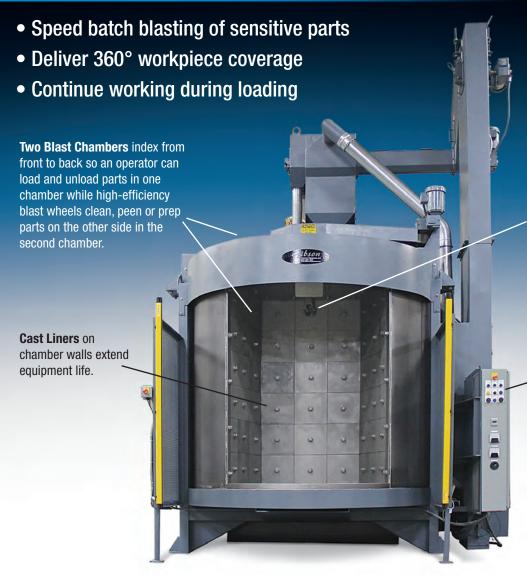
Motor-Driven Shaft spins workpiece fixtures for even, 360° exposure of part surfaces.
